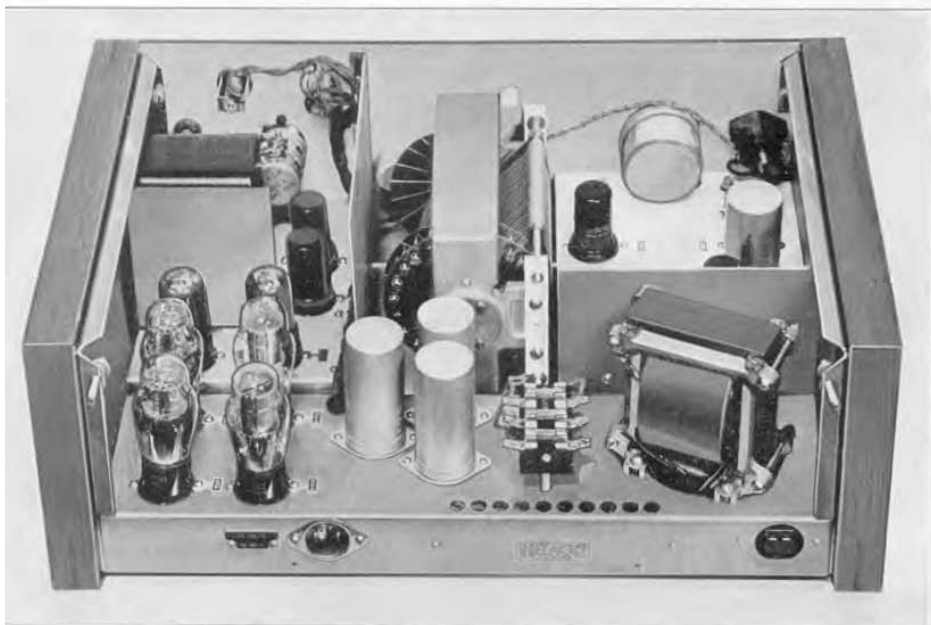
FIGURE 2. Rear view of the oscillator with dust cover removed. Note that tubes and fuses are easily accessible.
